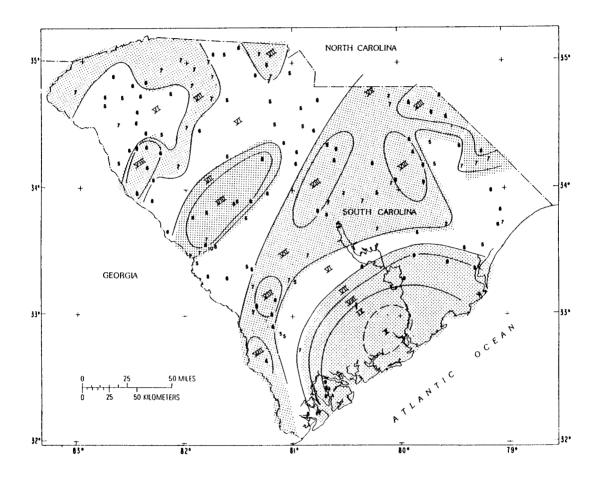
Figure 3: Detailed MM intensities and isoseismals from the 1886 Charleston, South Carolina, earthquake (after Bollinger, 1977). Areas with MMI≥VII are shown hatched.
