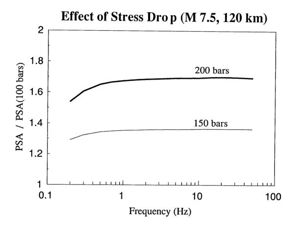
Figure 4: Ratio of spectral acceleration for 150 and 200 bars to 100 bars, for M=7.5 and R=120 km.
