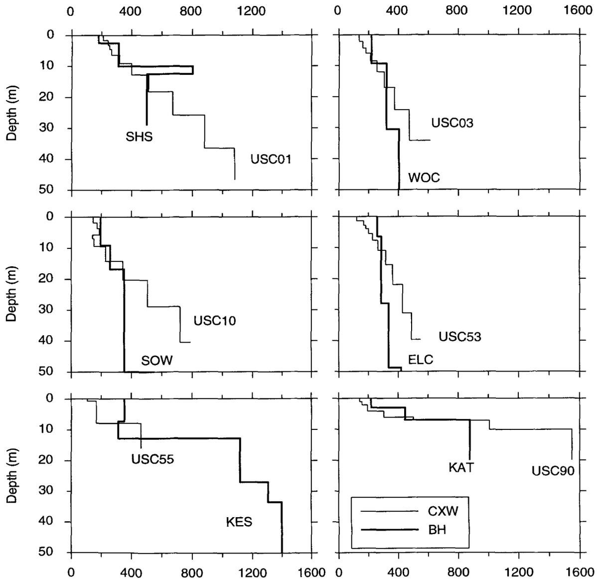
▲ **Figure 5** (corrected). Shear-wave velocity profiles obtained from the CXW method at six USC sites (thin lines), compared with velocities from downhole velocity profiles in boreholes drilled at or near the USC sites (thick lines).
