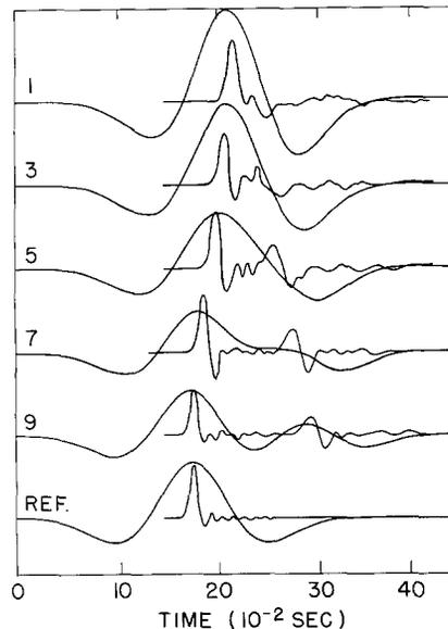
FIG. 3. Computed seismograms at selected sites in model 1. Reference trace is surface motion for a model without topographic relief. Time scale is based on assumed shear velocity of 500 m/sec.
