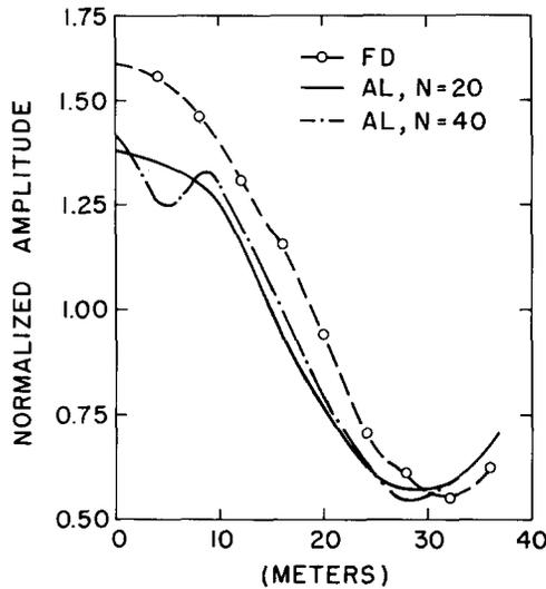
FIG. 2. Comparison of finite difference (FD) and Aki-Larner (AL) results for model 1 at a frequency of 5 Hz (assuming shear velocity of 500 m/sec).  $N$  is the number of scattering orders used in the AL method. The abscissa is horizontal distance from the center of the hill.
