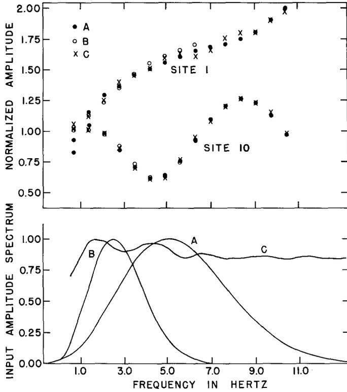
FIG. 4. (lower) Amplitude spectrum for three inputs to model 1. Shear velocity assumed to be 500 m/sec. (upper) Resulting spectral ratios, normalized to surface motion obtained if no topography were present, at sites 1 and 10.
