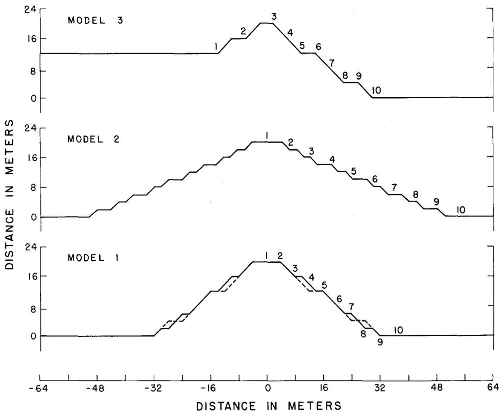
FIG. 1. Three topographic models used in the calculations. Numbers indicate spatial locations at which spectral ratios were formed. *Dashed lines* in model 1 indicate a configuration used in a run with grid spacing twice that of the *solid line* run.
