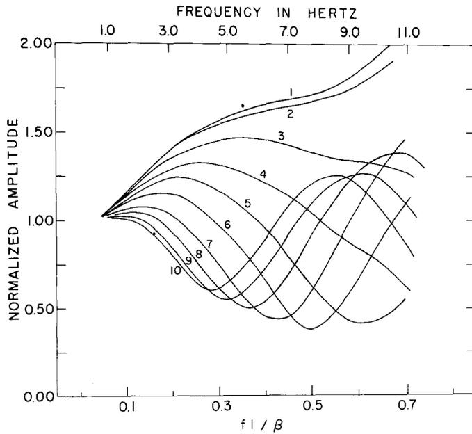
FIG. 5. Spectral ratio results for model 1 at various localities along the surface. Upper frequency scales represent assumed shear velocity of 500 m/sec.
